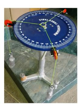
Apparatus consists of a circular aluminium disc of 40cm diameter, graduated in 360<sup>0</sup>. Apparatus is supplied complete with leveling screws, clamping device to fix the table at any desired angle, five sliding clamp pulleys, central ring, string and five sets of iron nickled slotted weights (each set containing nine weights and one hanger of 50 gm each).
